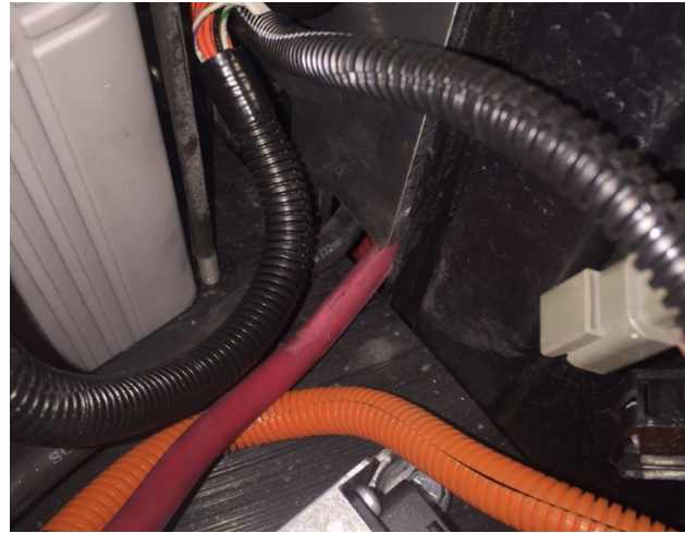
Fig. 26- Cable routing from battery pack
