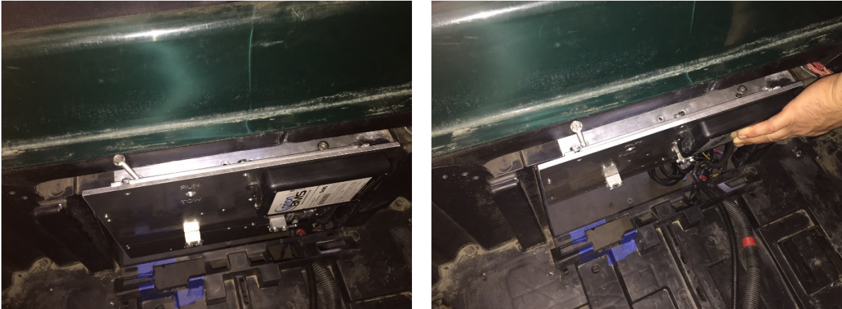
Fig. 19 – Fully assembled controller plate installed
