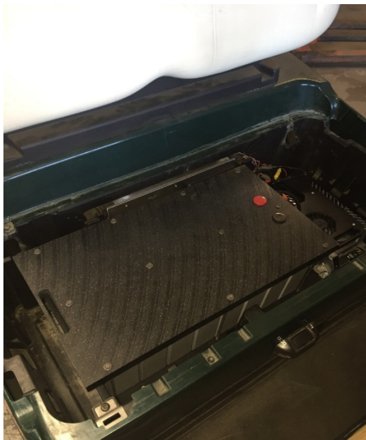
Fig. 20-Lithium battery pack installed into golf car
