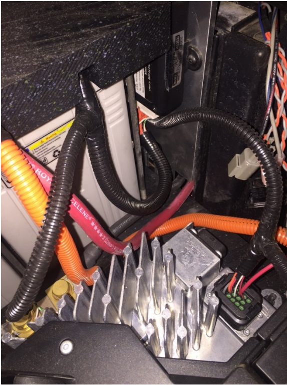
Fig. 26- Cable routing from battery pack
